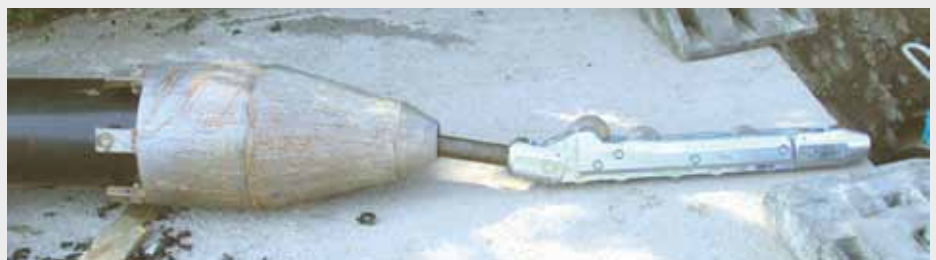
Mühlethurnen: The new roller cutter DN 100 mm (4") with expander cone Ø 324 mm (12.75") and HDPE pipe OD 250 mm (10").
